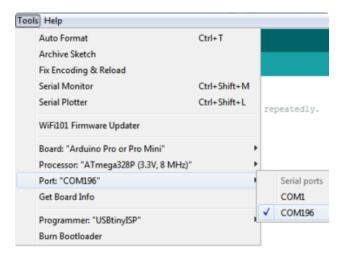
Then from Tools select the Port to be the serial port of the Feather. See above for how to find your COM/Serial port!
