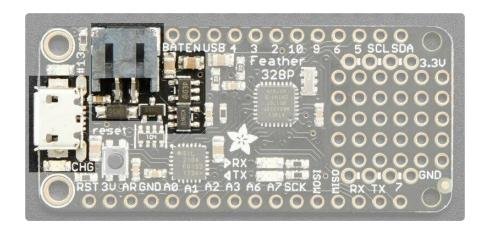
The above shows the Micro USB jack (left), LiPoly JST jack (top left), as well as the 3.3V regulator (to the right of the JST) and changeover diode + FET (just below the JST jack) and the LiPoly charging circuitry (below the regulator).
