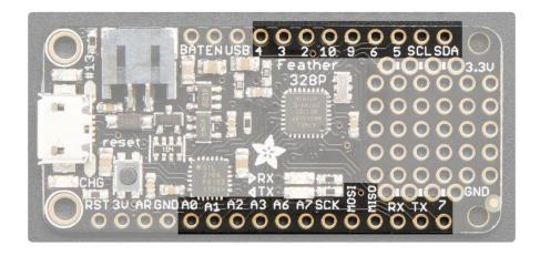
This is the general purpose I/O pin set for the microcontroller. All logic is 3.3V
