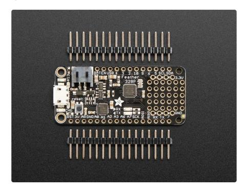
With this Feather we're getting a little nostalgic for the ATmega328P - the classic 'Arduino' chip - with this Adafruit Feather 328P running a 3.3V and 8 MHz. Feather is the new development board from Adafruit, and like it's namesake it is thin, light, and lets you fly! We designed Feather to be a new standard for portable microcontroller cores. We have other boards in the Feather family, check'em out here. (https://adafru.it/I7B)
