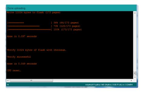
After uploading, you may see a message saying "Disk Not Ejected Properly" about the ...BOOT drive. You can ignore that message: it's an artifact of how the bootloader and uploading work.
