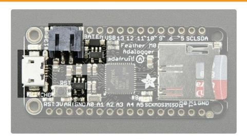
The above shows the Micro USB jack (left), LiPoly JST jack (top left), as well as the 3.3V regulator and changeover diode (just to the right of the JST jack) and the LiPoly charging circuitry (to the right of the Reset button).
