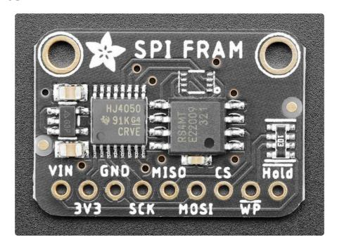
The FRAM is the chonky chip to the right of the center of the board. Along the bottom we have power and interface pins.
