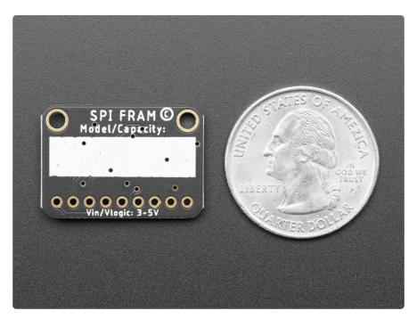
These particular FRAM chips have 2 or 4 Megabits (256 or 512 KBytes) of storage, interfaces using SPI, and can run at up to 40 MHz clock rates. Each byte can be read and written instantaneously (like SRAM) but will keep the memory for 95 years at room temperature.
