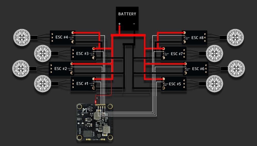
IMPORTANT: PLEASE DO NOT CONNECT THE 5V OUT OF THE ESC TO FC, IT WILL CAUSE THE ESC/FC TO BURN
