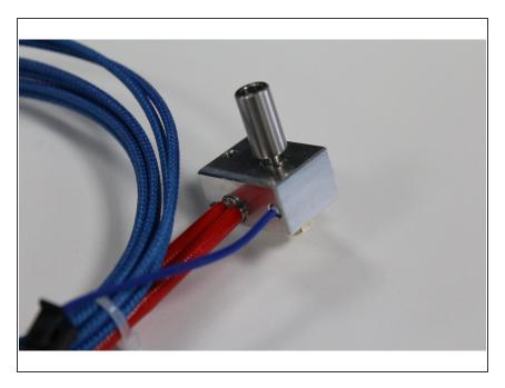
Before moving on, gently tug on your thermistor and heater cartridge wires. We don't want them slipping out during a print!
