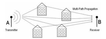
In a multipath rich conditions is it recommended that each pMDDL end have a pair (2) of omni directional antennas that have at least half-wavelength distance between them. A set of (4) Omnidirectional antennas is good for a pair of pMDDL radios.
