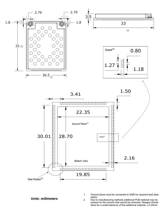
Drawing 3-1: pMDDL OEM Mechanical
