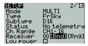
Long press the MDL button to enter the model settings, select MULTI on the SETUP page, and select the desired protocol in the sub-options. The system will automatically turn on the corresponding RF module according to the RF protocol you selected.
