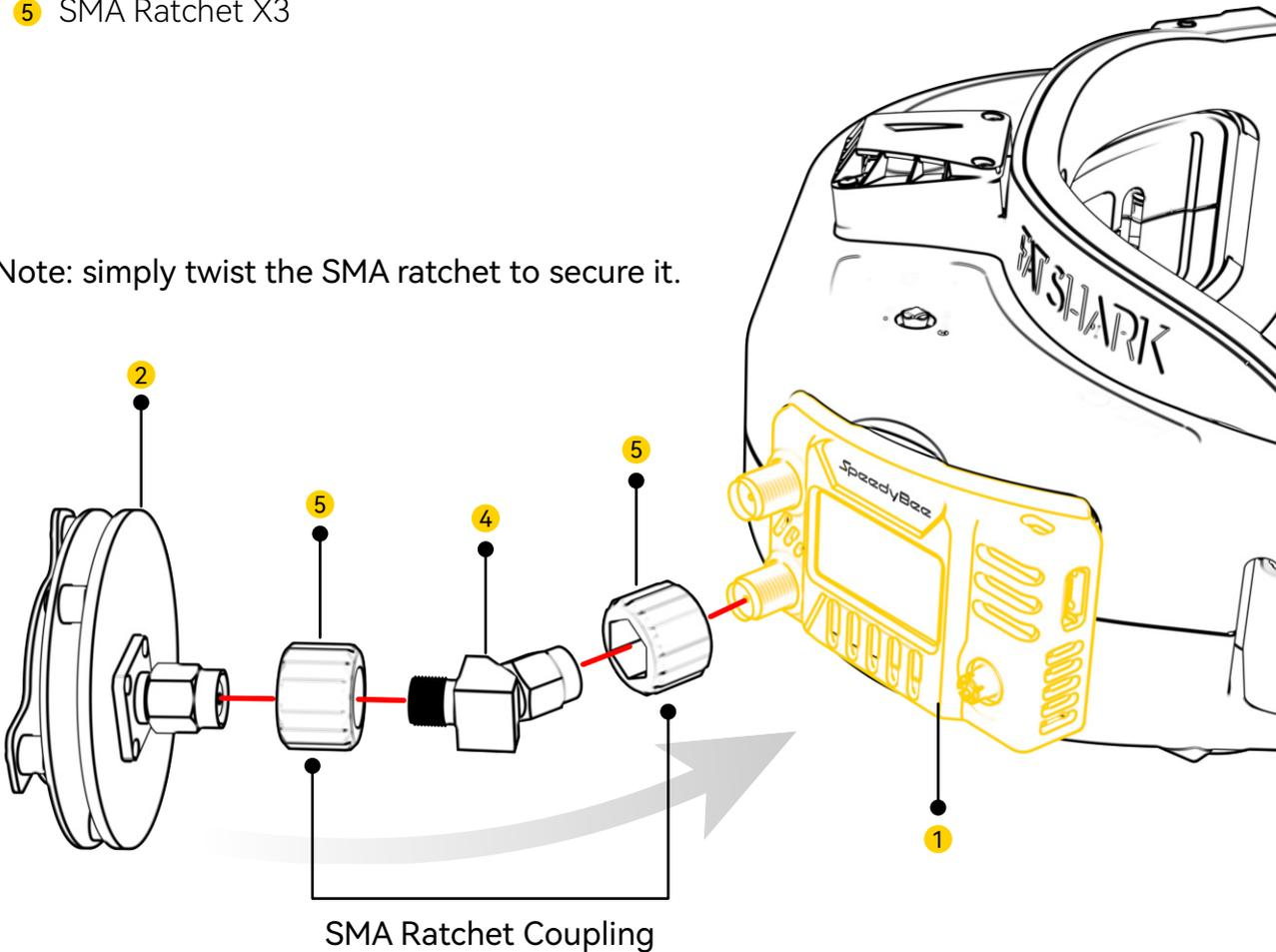
\*Note: simply twist the SMA ratchet to secure it.
