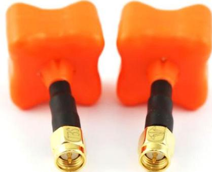
RP-SMA - center-pin (LHCP antenna)
