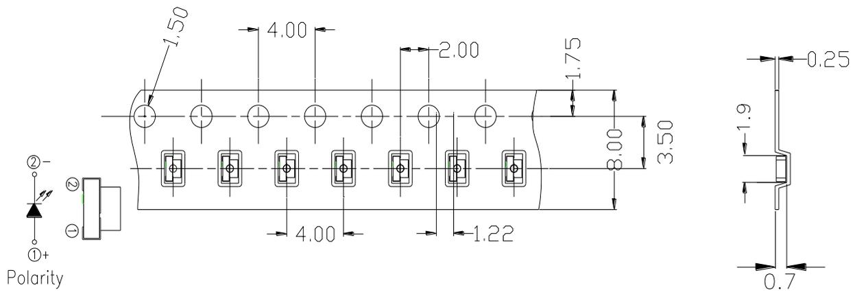
Note: The tolerances unless mentioned is  $\pm 0.1\text{mm}$  ,Unit = mm
