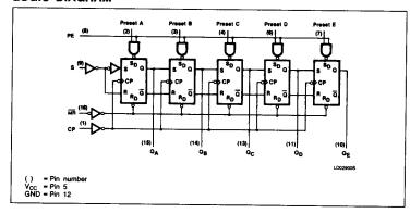
Each flip-flop has asynchronous set inputs, allowing them to be independently set HIGH. The set inputs are controlled by a common active HIGH Preset Enable (PE) input. The PE input is not buffered, and care must be taken not to overload the driving element. When the PE is HIGH, a HIGH on the Preset (A-E) inputs will set the associated flip-flops HIGH. A LOW on the A - E inputs will cause "no change" in the appropriate flip-flops.
