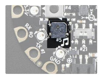
You can make your circuit playground sing with the built in buzzer. This is a miniature magnetic speaker connected to digital pin #5 with a transistor driver. You can use PWM at varying frequencies to make basic tones.
