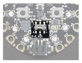
There is a single slide switch near the center of the Circuit Playground. It is connected to digital #21 and will read LOW when slid to the left, and HIGH when in the right hand position
