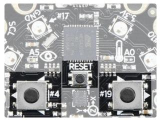
This small button in the center of the board is for Resetting the board. You can use this button to restart or reset the CPC.
