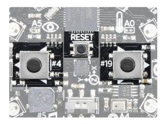
There are two large buttons, connected to digital #19 (Left) and #5 (Right) each. These are pulled to ground when not pressed, and connected to 3.3V when pressed, so they read HIGH.
