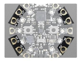
Of the 14 pads, you get a wide range of power pins, I2C, UART, Analog In, Digital In/Out and PWMt.
