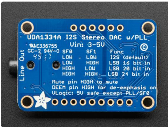
**SF0** and **SF1** are used to set the input data format. By default both are pulled Low for I2S but you can change them around for alternate formats.
