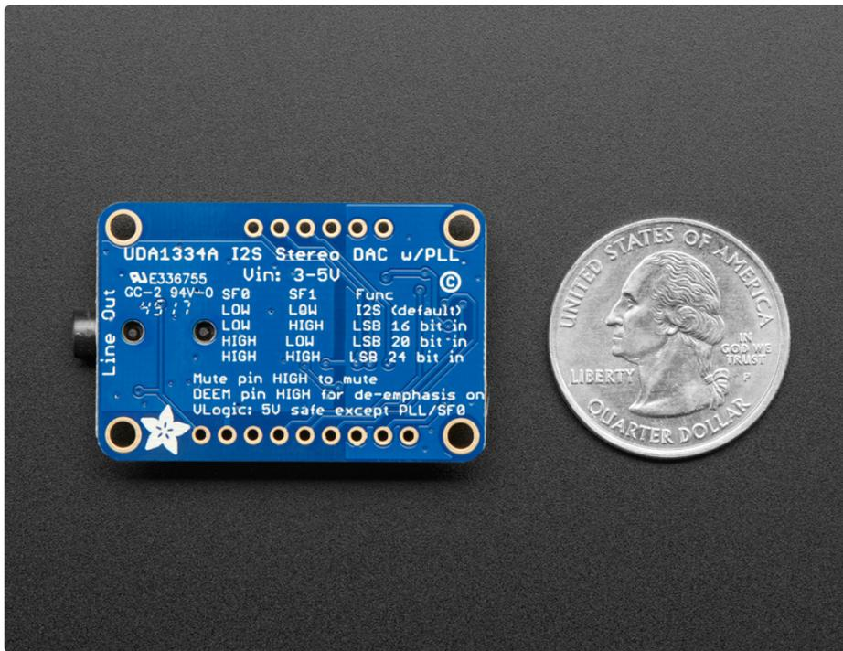
We put in plenty of ferrite beads, a low-dropout regulator, and the recommended band-pass filter so you get a very nice clean output. With a sine-wave generator we swept through 20-20KHz and saw no
