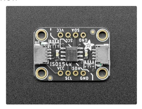
Sometimes you'll find yourself with an I2C bus controller on one side, and an I2C bus device on the other and you gotta keep em (electrically) separated (https://adafru.it/QsD). Maybe because one is Earth-grounded, maybe because you've got some funky power monitoring setup, maybe you want to reduce noise.
