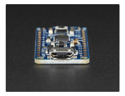
Like the Trinket, it has onboard USB bootloading support - we opted for a MicroUSB jack this time. We also added Optiboot support, so you can either program your Pro Trinket over USB or with a FTDI cable just like the Pro Mini and friends.
