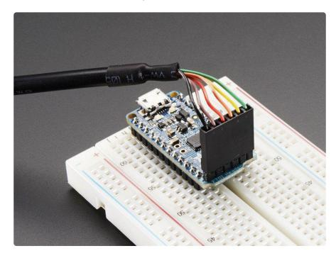
The Pro Trinket PCB measures only  $1.5" \times 0.7" \times 0.2"$  (without headers) but packs the same capability as an Arduino UNO. So it's great once you've finished up a prototype on an official Arduino UNO and want to make the project smaller.
