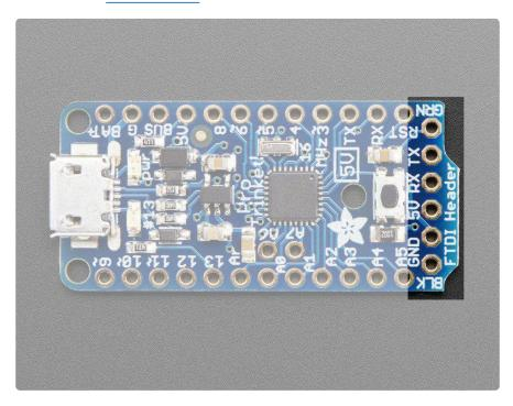
The bootloader on Pro Trinket is dual USB & FTDI "optiboot" so you can use either the USB port or the FTDI breakout to upload. However, only the FTDI port allows you to use Serial debugging. So it's a bit of a tradeoff - USB is inexpensive, built-in but requires a button press to start & there's no debugging, FTDI requires an extra cable but has auto-reset and debug console.
