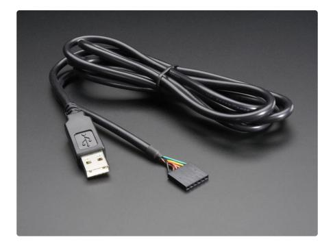
For beginners, we suggest using an FTDI cable for programming and debugging, especially if you aren't simply porting an existing Arduino project to Pro Trinket. Much like many Arduino-compatibles, there's a header for connecting a <u>'classic' FTDI cable</u> ( https://adafru.it/dNN) or FTDI friend. (https://adafru.it/dQa)
