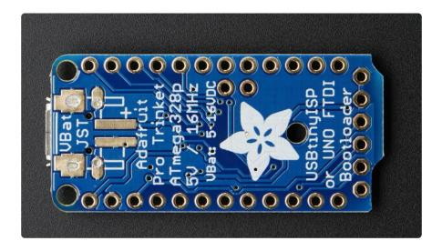
On the bottom there's a spot for a <u>2-pin JST-PH connector</u> (http://adafru.it/1769). this is optional and can be soldered on by hand. It will let you use a lipoly or <u>AAA battery</u> <u>pack</u> (http://adafru.it/727) or <u>a JST cable</u> (https://adafru.it/drM) for other power input. It's connected to the GND and VBAT pins
