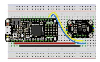
Board 3V to sensor VIN (red wire) Board GND to sensor GND (black wire) Board SCL to sensor SCL (yellow wire) Board SDA to sensor SDA (blue wire)
