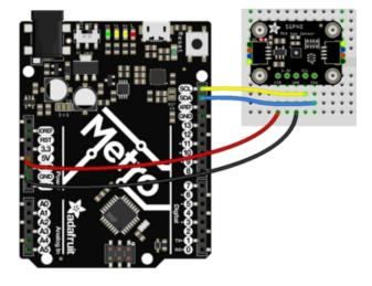
Connect board VIN (red wire) to Arduino 5V if you are running a 5V Arduino (Uno, etc.). If your Arduino is 3V, connect to that instead.
