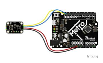
Connect board VIN (red wire) to Arduino 5V if you are running a 5V Arduino (Uno, etc.). If your Arduino is 3V, connect to that instead.
