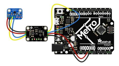
Simply add connections for VIN, GND, SCL, and SDA between the SGP40 and SHT31 as seen above. Alternately the SHT31 can be wired directly to the Metro's I2C connections.
