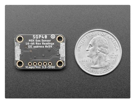
The SGP40 has a 'standard' hot-plate MOX sensor, as well as a small microcontroller that controls power to the plate, reads the analog voltage and provides an I2C interface to read from. Unlike the CCS811, this sensor does not require I2C clock stretching. We currently have an Arduino library with examples of reading the raw value and also running the Sensirion algorithm to calculate VOC index (https://adafru.it/PaX) as well as a CircuitPython / Python library (https://adafru.it/PBZ).
