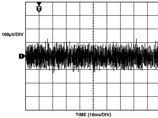
Figure 16. ADR381 Typical Noise Voltage, 10 Hz to 10 kHz
