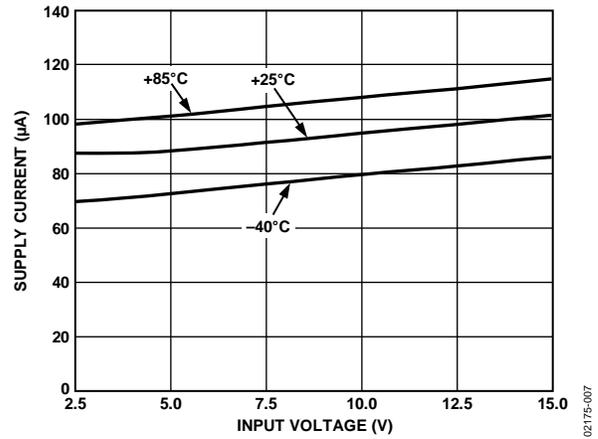
Figure 7. ADR381 Supply Current vs. Input Voltage
