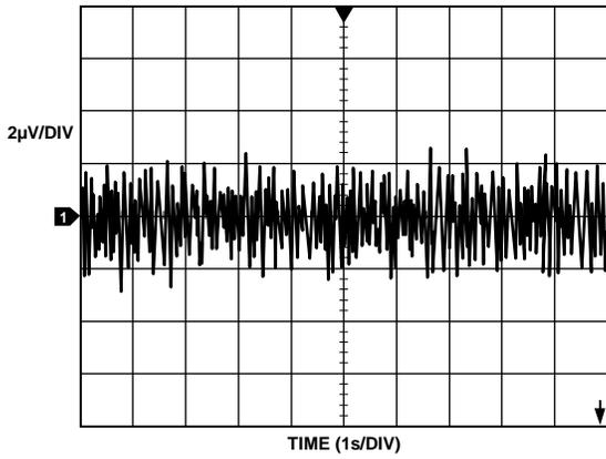
Figure 15. ADR381 Typical Noise Voltage, 0.1 Hz to 10 Hz
