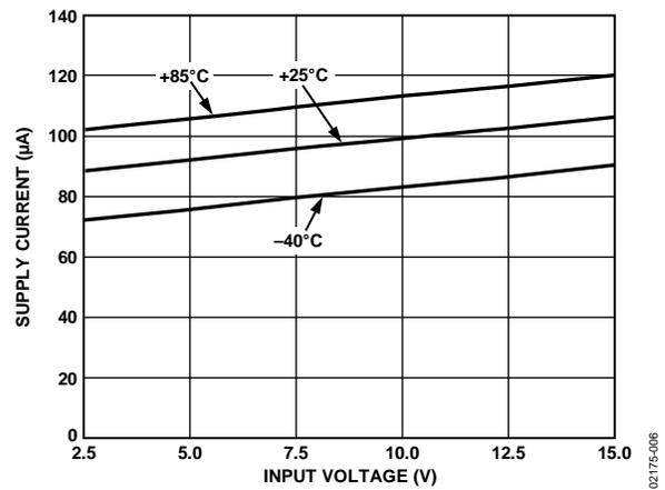
Figure 6. ADR380 Supply Current vs. Input Voltage
