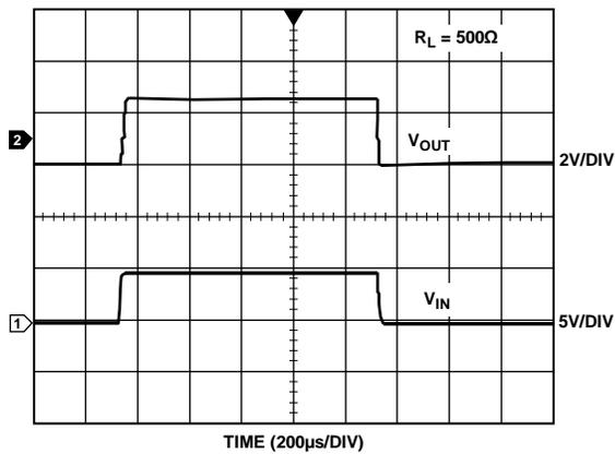
Figure 22. ADR381 Turn-On/Turn-Off Response at 5 V
