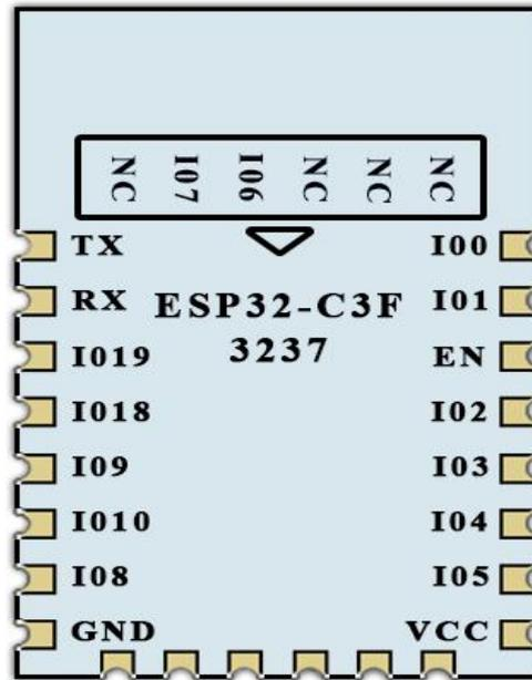
ESP32-C3F Diagram of Pin
