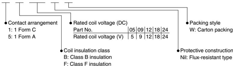
Notes: 1. The "W" at the end of the part No. only appears on the inner and outer packaging. It does not appear on the relay itself.
