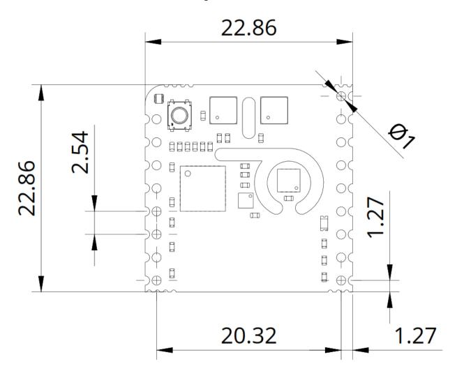
The Nicla Sense Env does not have mounting holes for mechanical fixing. The slots found in the board were placed because of the board's sensor requirements and specifications.
