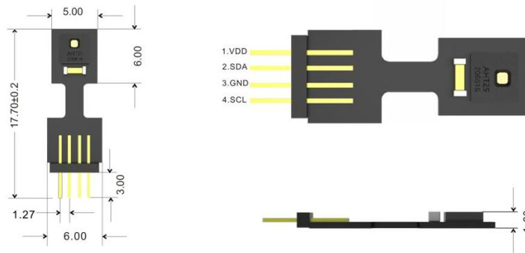
Figure 12. AHT25 sensor encapsulation (unit: mm unmarked tolerance: ± 0.1mm)
