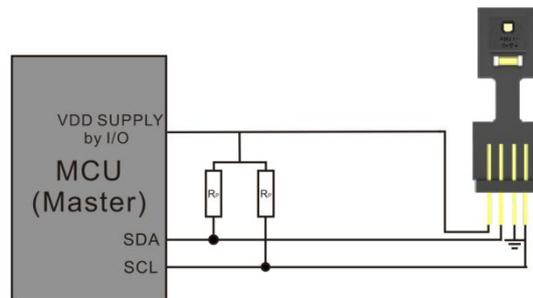
Figure 8. Typical application circuit
