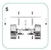
Fix the rear spoiler to the baseplate with the help of brass standoff. Take out standoff and screws from the bag label "For Spoiler
