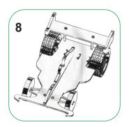
Finally make the connections of the motors, Li-ion charger to the remote & place the Li-ion cell and drive the car with the remote
