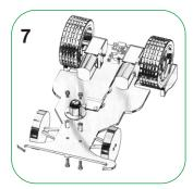
Mount the small castor wheel below the front spoiler. Take out standoff and screws from the bag label "for castor"
