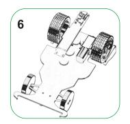
Place the SmartElex 1S 18650 Li-ion charger on the baseplate by using 3M DST pads as shown in the fig.
