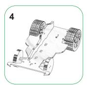
Snap the front spoiler to the baseplate as shown in the fig.
