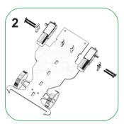
Fix the BO motors to the baseplate with the help of the motor clamps and screws as shown in fig. Take out Motor clamps & screws from the bag label "for motor".
