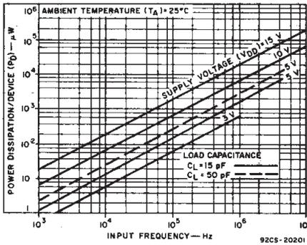
Fig. 8 — Typical power dissipation vs. frequency.
