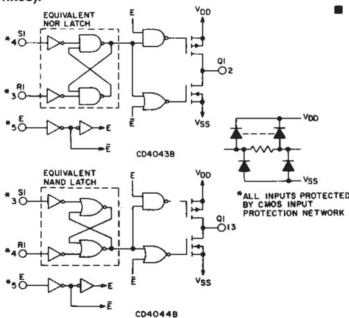
Fig. 1 - Logic diagrams.
