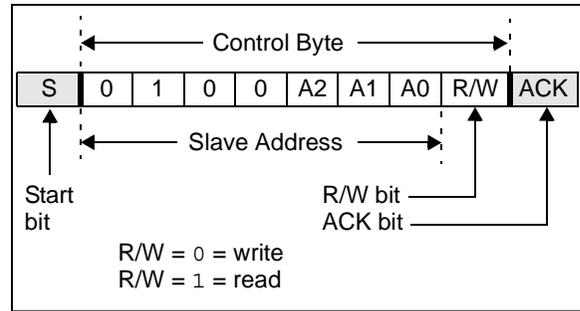
**FIGURE 1-3: SPI™ CONTROL BYTE FORMAT**
