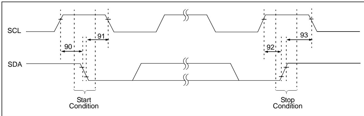
**FIGURE 2-4: I<sup>2</sup>C™ BUS DATA TIMING**
