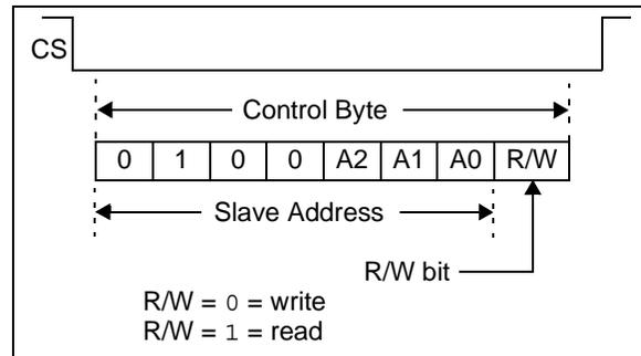
**FIGURE 1-4: I<sup>2</sup>C™ ADDRESSING REGISTERS**
