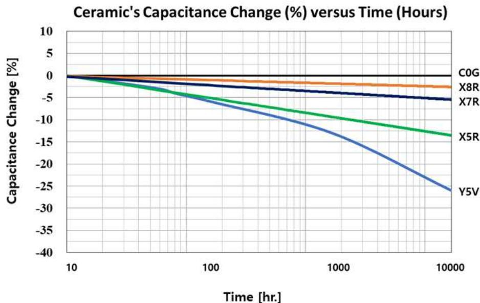
The capacitance value can be restored ( a.k.a. 'de-aged' ) by exposing the component to elevated temperatures approaching its Curie Temperature ( approximately 120°C ). This 'deaging' can occur during the component's solder-assembly onto the PCB, during life or temperature cycle testing., or by ' baking ' at 150°C for about 1 hour.
