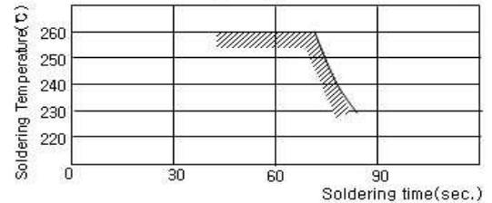
In case of repeated soldering, the accumulated soldering time must be within the range shown above.
