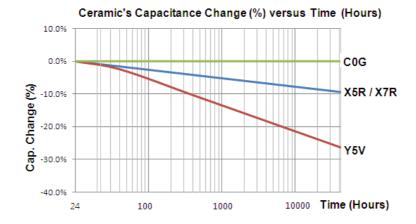
The capacitance value can be restored (a.k.a. 'de-aged') by exposing the component to elevated temperatures approaching its Curie Temperature (approximately  $120\,^{\circ}$ C). This 'deaging' can occur during the component's solder-assembly onto the PCB, during life or temperature cycle testing., or by 'baking' at  $150\,^{\circ}$ C for about 1 hour.
