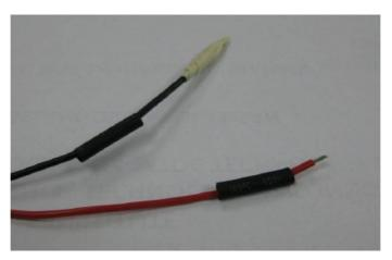
4. Solder the wire to Dean-T connector. Be careful while soldering and make sure the polarity is correct.
