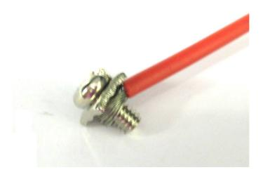
4. Put back the screw into terminal block and tighten the screw.
