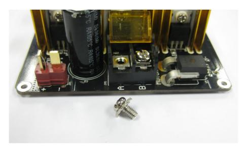
3. Wrap the wire of DC motor around the screw.
