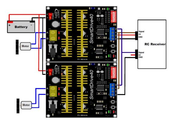
2. Set the DIP Switch to operate in RC mode. Driver for left motor must be set as left mix mode and driver for right motor must be set as right mix mode. Exponential can be turned on or off for both motor, but both motor must have the same exponential setting. MCU mode should be turned off for both motor.
