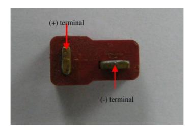
2. Cut and remove the wire insulator. If user needs to solder the wire directly from battery to Dean-T connector, solder **one terminal at a time** and leave another one wrapped.
