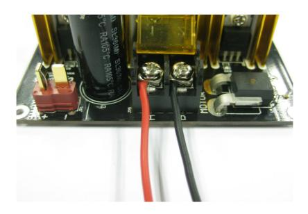
6. This is an example connection of DC motor via terminal block.
