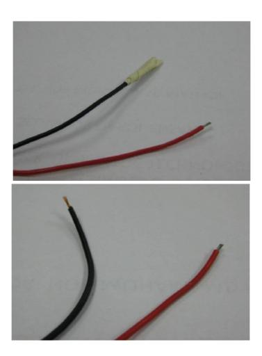
3. Cut the shrinking tube to ~2cm each. Slide in the shrinking tube into the wire. The shrinking tube is used to protect the connection at the Dean-T terminal.
