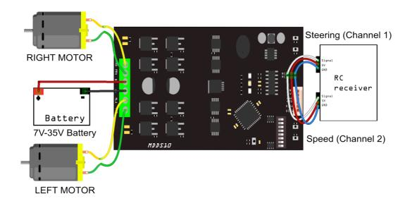
RC Mode with Microcontroller (Independent Both), DIP switch
