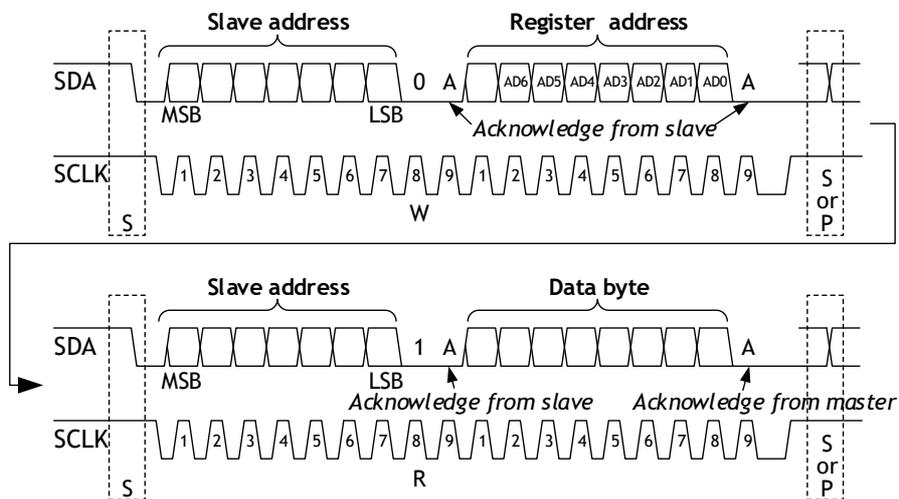
Figure 13: I<sup>2</sup>C Auto-Increment Read Operation
