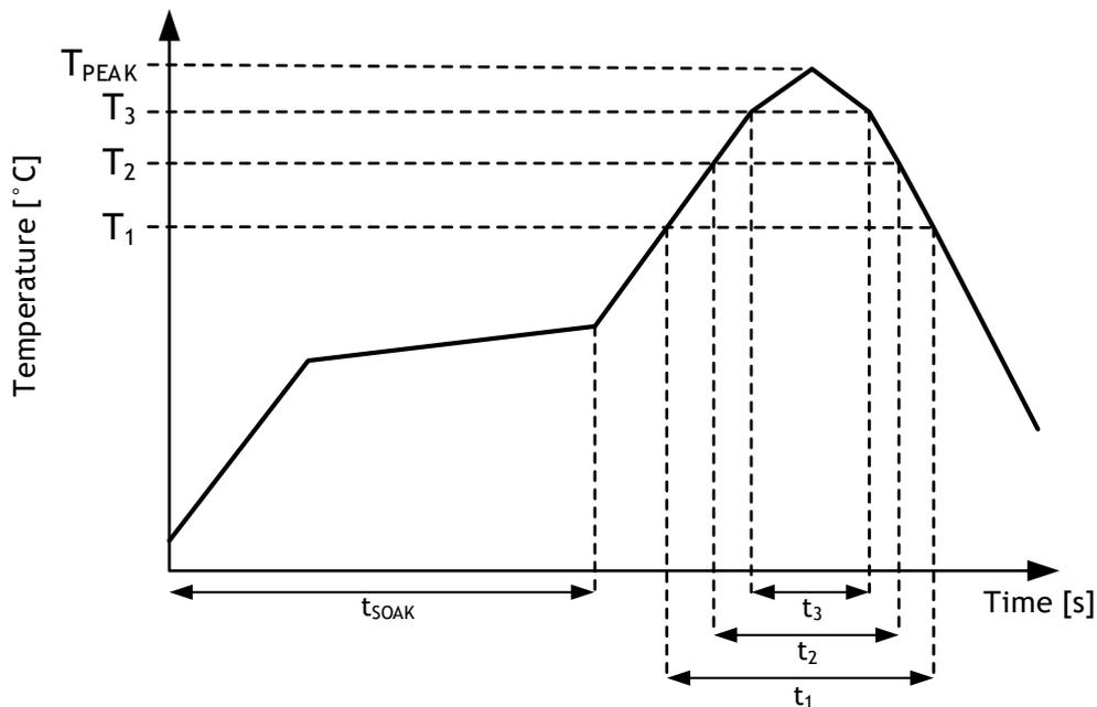
The detailed settings for the reflow profile are shown in the table below.
