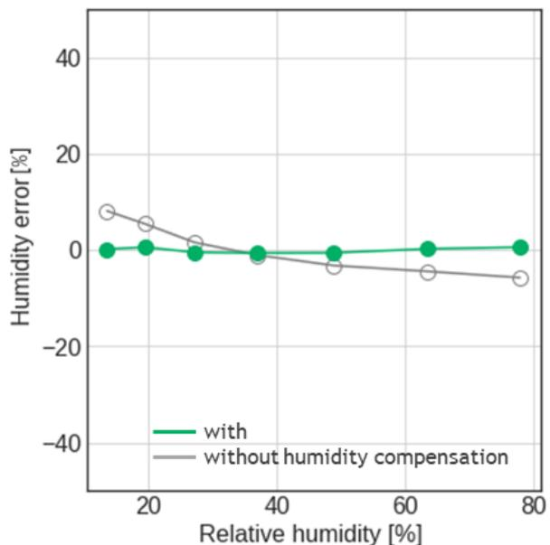
**Note:** Unless otherwise stated, the humidity compensation discussed in this section works per default for all output signals except for sensor raw signals.
