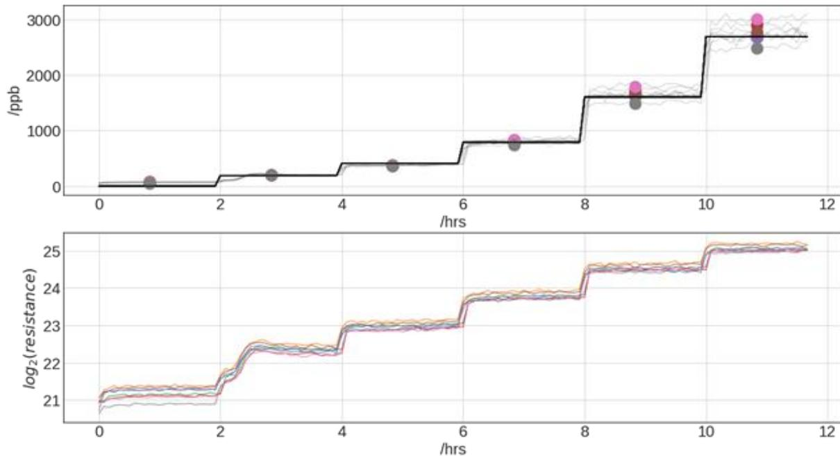
**Note:** Due to the nature of sensor raw resistance values, these signals are not conditioned, i.e. not compensated for drift, ageing or cross-sensitivity (interference of background gases including humidity).
