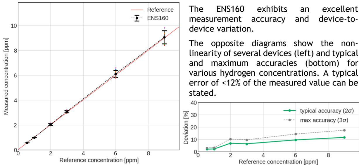
The ENS160 exhibits an excellent measurement accuracy and device-to-device variation.
