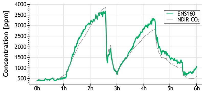
The ENS160 reverses the proportional correlation of VOCs and CO<sub>2</sub>, by providing a standardized output signal in ppmCO<sub>2</sub>-equivalents from measured VOCs plus hydrogen, thereby adhering to today's CO<sub>2</sub>-standards, as shown opposite: ENS160-based equivalent CO<sub>2</sub> estimate vs. CO<sub>2</sub>, detected by an NDIR-sensor during two consecutive meeting sessions, interrupted by a lunch-break.
