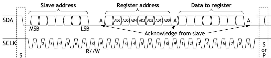
Figure 15: I<sup>2</sup>C Auto-Increment Write Operation
