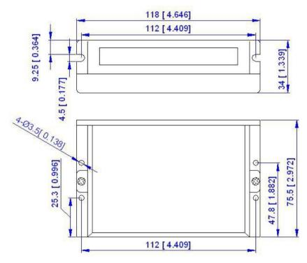
Figure 1: Mechanical specifications
