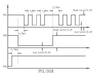
Figure 10: Sequence chart of control signals
