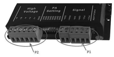
The DM556T has two connector blocks P1&P2 (see above picture). P1 is for control signals connections, and P2 is for power and motor connections. The following tables are brief descriptions of the two connectors. More detailed descriptions of the pins and related issues are presented in section 4, 5, 9.
