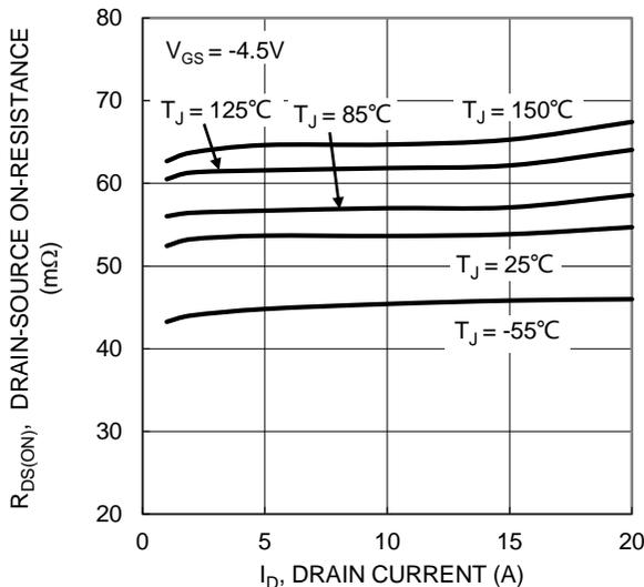
Figure 17. Typical On-Resistance vs. Drain Current and Temperature
