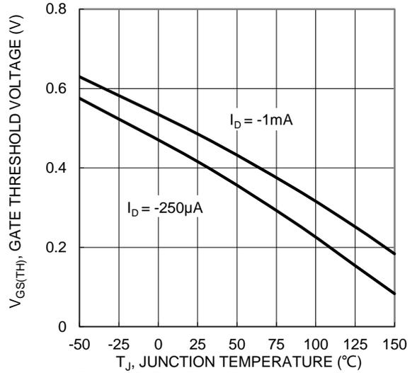
Figure 20. Gate Threshold Variation vs. Junction Temperature
