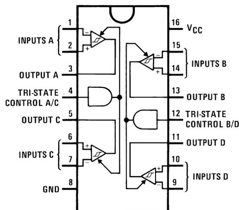
Figure 1. Dual-In-Line Package
