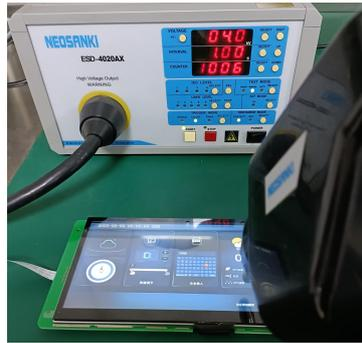
3.1 Electrostatic discharge test
