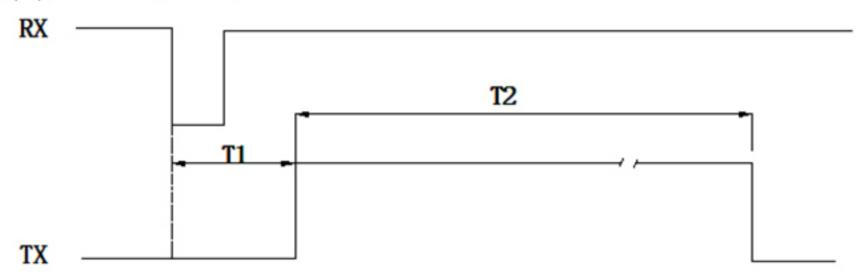
Remark: T1=10~17ms; Flat object T2=0.18~35ms(PWM High level pulse width timing)
