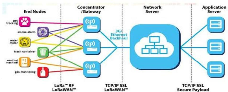
The complete LoraWan network system consists of: nodes, gateways, Lora NetWork Server, and application servers. The nodes are generally designed by LORA chips; the gateway is designed by SX1301 provided by semtech; the Lora NetWork Server currently has open source loraserver or commercial TTN (The ThingsNetwork), users can build it by themselves; the application server is designed and developed by users, mainly used for exchanging application data with Lora NetWork Server.
