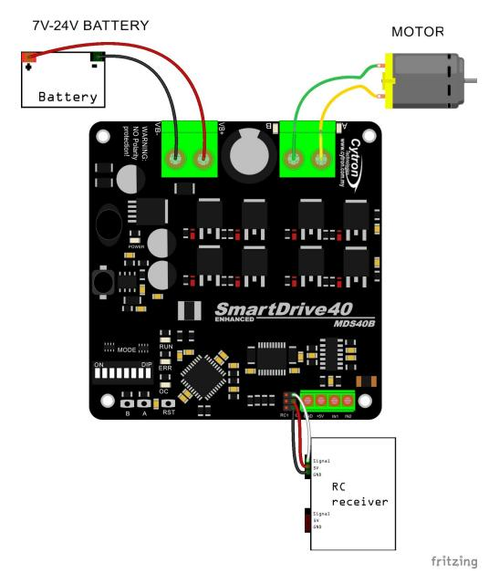
RC Mode with RC Transmitter/Receiver (Mixed Right), DIP switch
