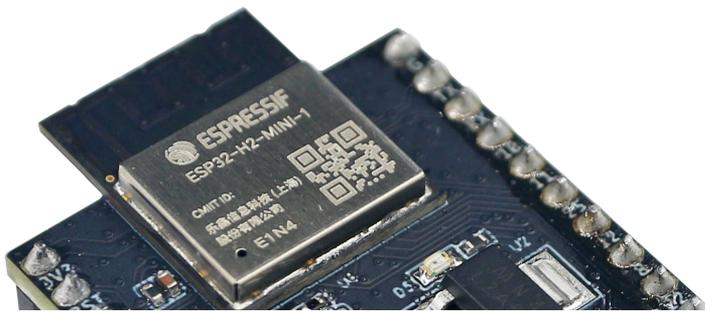
*ESP32-H2-DevKitM-1 (with ESP32-H2-MINI-1 on board)*
