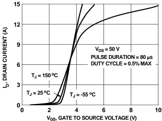
Figure 5. Transfer Characteristics
