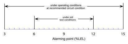
Expected performance of LP gas detectors using LPM2610 and 9% LEL alarming point
