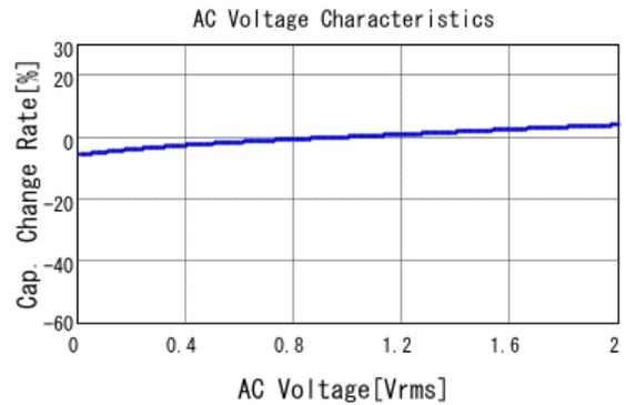
GCM155R71H104KE02 C-AC Voltage capchange, DC0V, 25.0d
