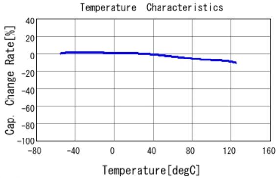
■ GCM155R71H333KE02 C-Temp. capchange, DC0.0V, AC1.0V<sub>rm</sub>
