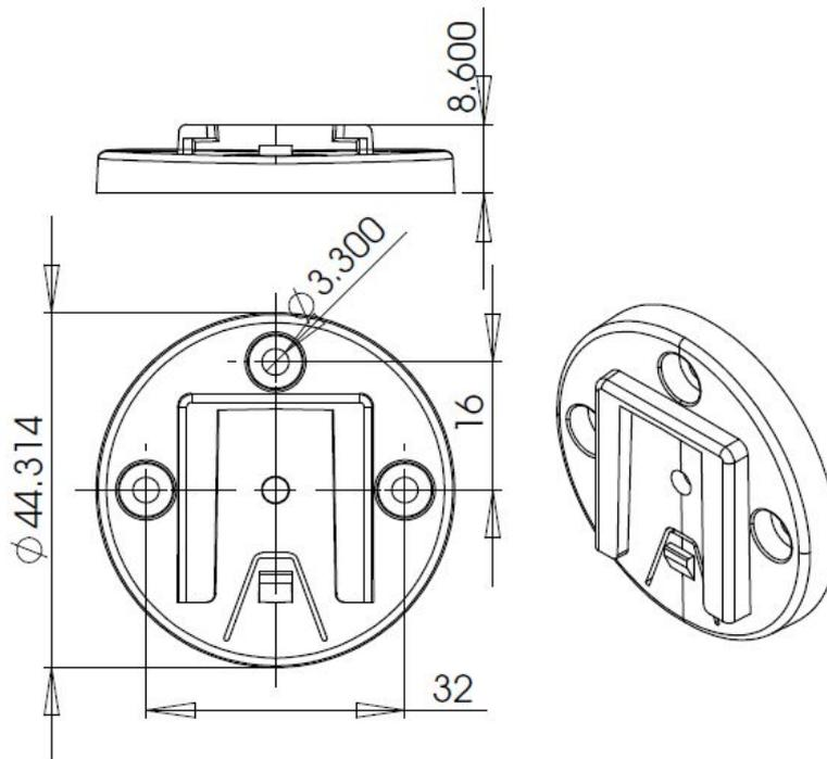
**8.4 G15 Rotatable Connect Dimensions (mm):**
