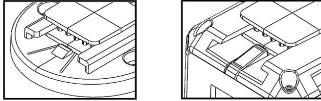
**Make sure all the connects are locked properly to the joint by the latch**
