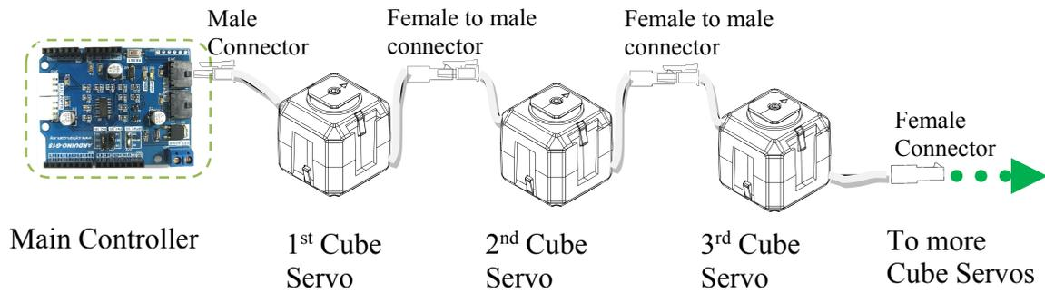
Figure above shows the daisy chain connection of G15 Cube Servo to create a servo network on a single power and communication line.
