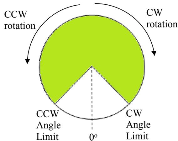
If the CW Angle Limit value is more than the CCW Angle Limit value, for example CW Angle = 350° and CCW Angle Limit = 10°, G15 servo will operate in shaded sector as shown in the figure below.
