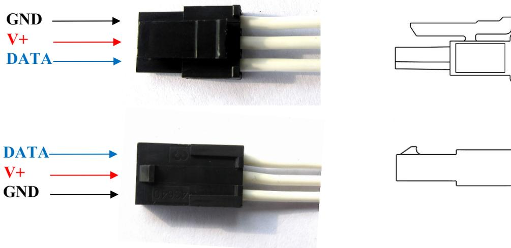
G15 Cube Servo uses high quality silicone rubber wire (22AWG) and Molex Micro-Fit connector with clip for the power and data line. Types of Connector for G15 Cube Servo are listed as in table below:
