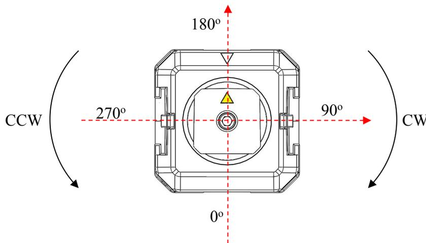
The GOAL POSITION is the destination position that G15 shaft will move to and positioned. G15 can be electrical positioned to any 360 degrees of position. The resolution of the positioning is 0.33°. The value of GOAL POSITION can be from 0 to 1087 which represent
