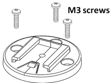
**External Joint can be screwed to customized part with M3 screws.**
