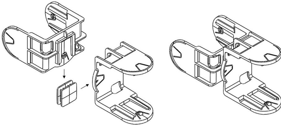
**U-Joint – Inter Connect – External Joint**
