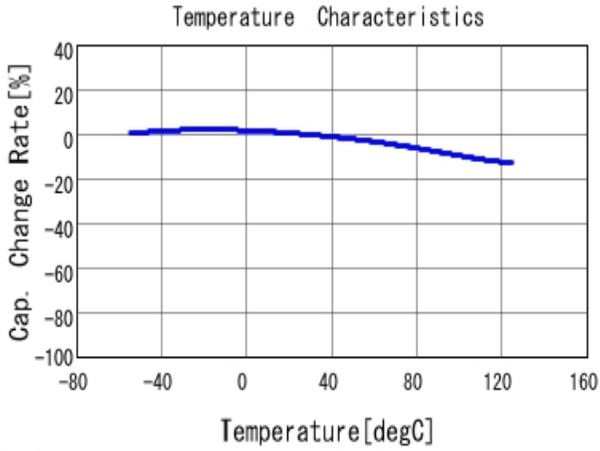
■ GRT155R71H104KE01 C-Temp. capchange, DC0.0V, AC1.0V<sub>r</sub>m
