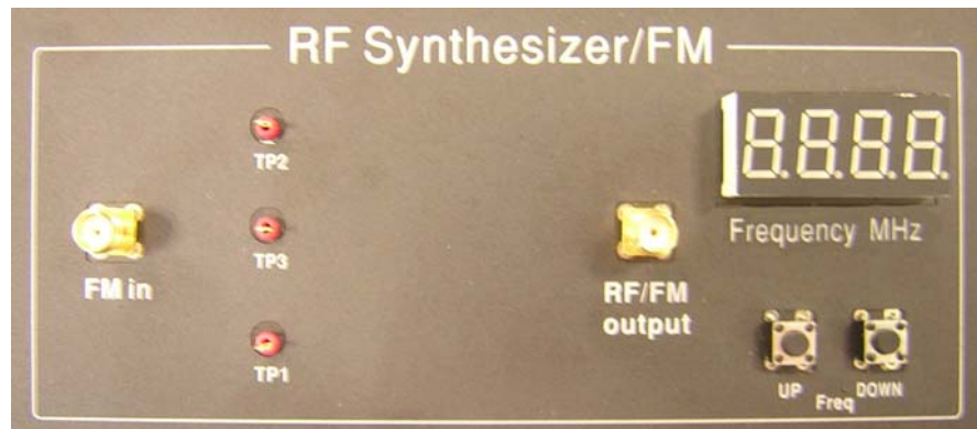
Figure A-5. RF Synthesizer/FM module
