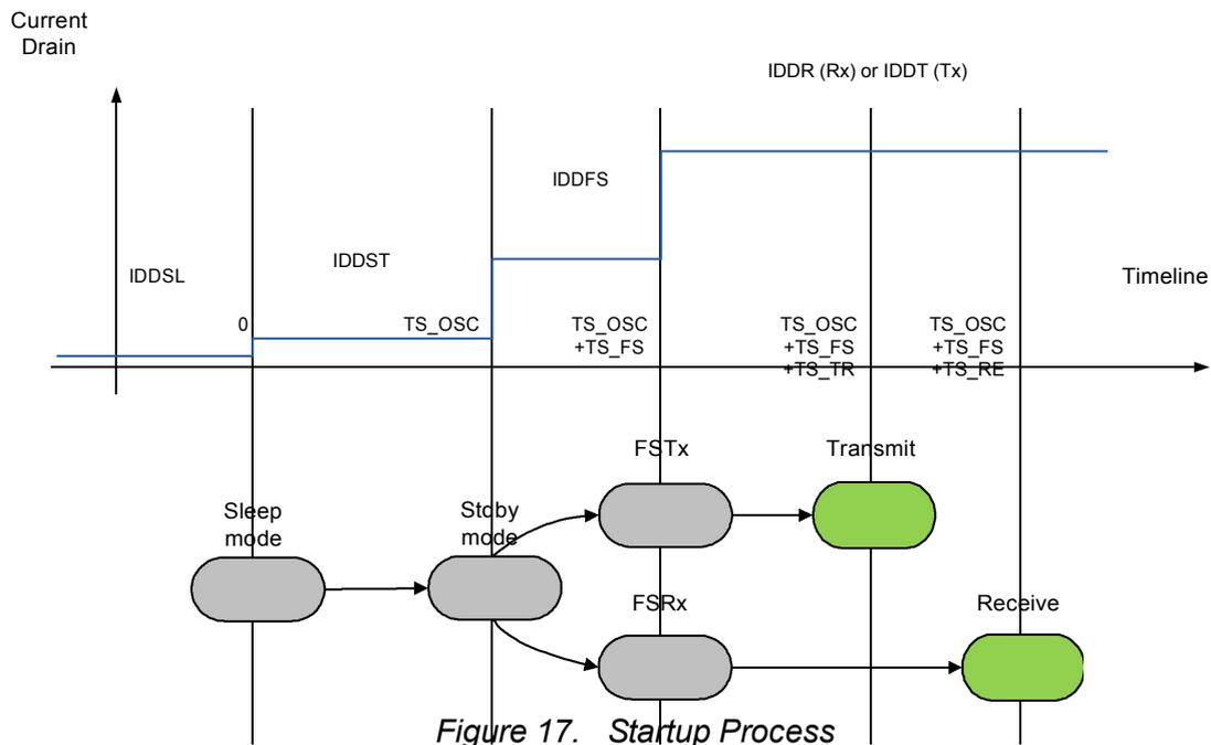
$TS\_OSC$  is the startup time of the crystal oscillator which depends on the electrical characteristics of the crystal.  $TS\_FS$  is the startup time of the PLL including systematic calibration of the VCO.
