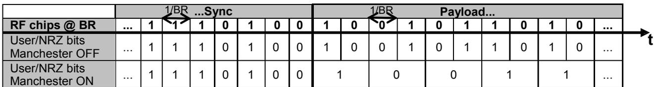
Figure 36. Manchester Encoding/Decoding
