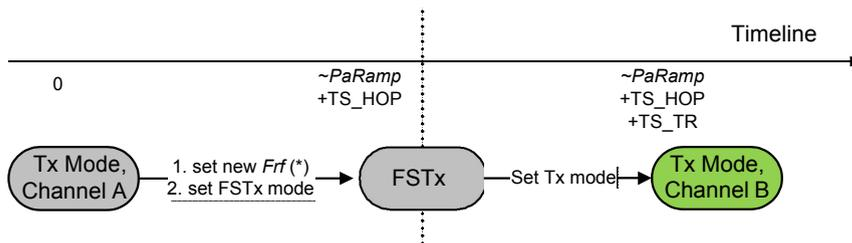
Figure 22. Transmitter Hopping
