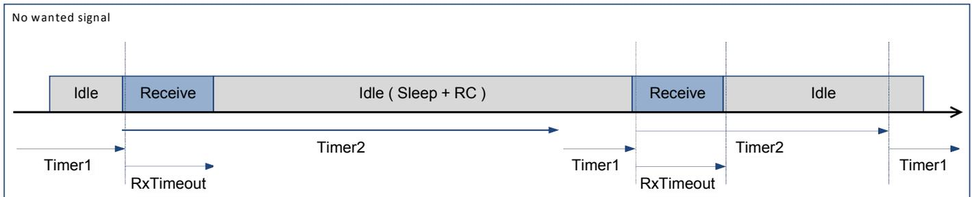
Figure 48. Listen Mode with no SyncAddress Detected
