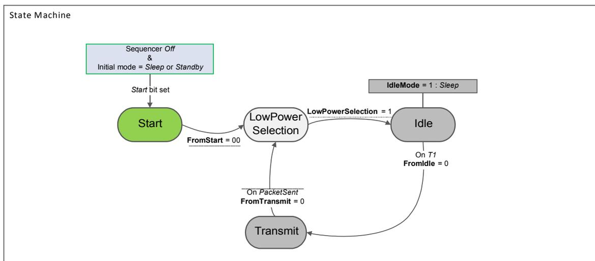
Figure 53. Beacon Mode State Machine
