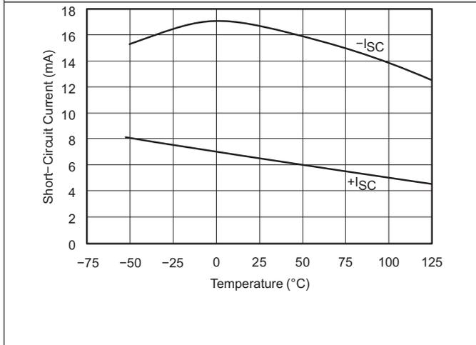
**Figure 15. Short Circuit Output Current vs Temperature**
