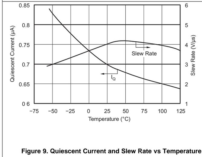
Figure 9. Quiescent Current and Slew Rate vs Temperature
