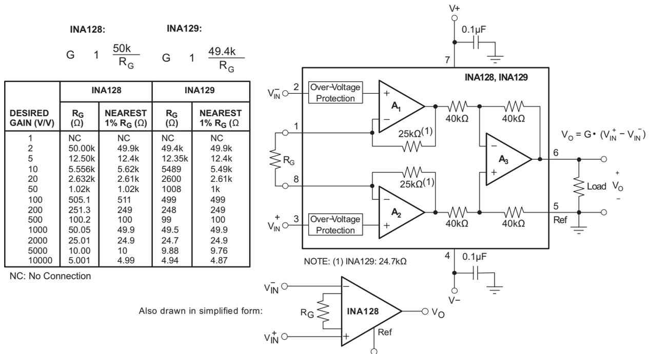
**Figure 24. Basic Connections**
