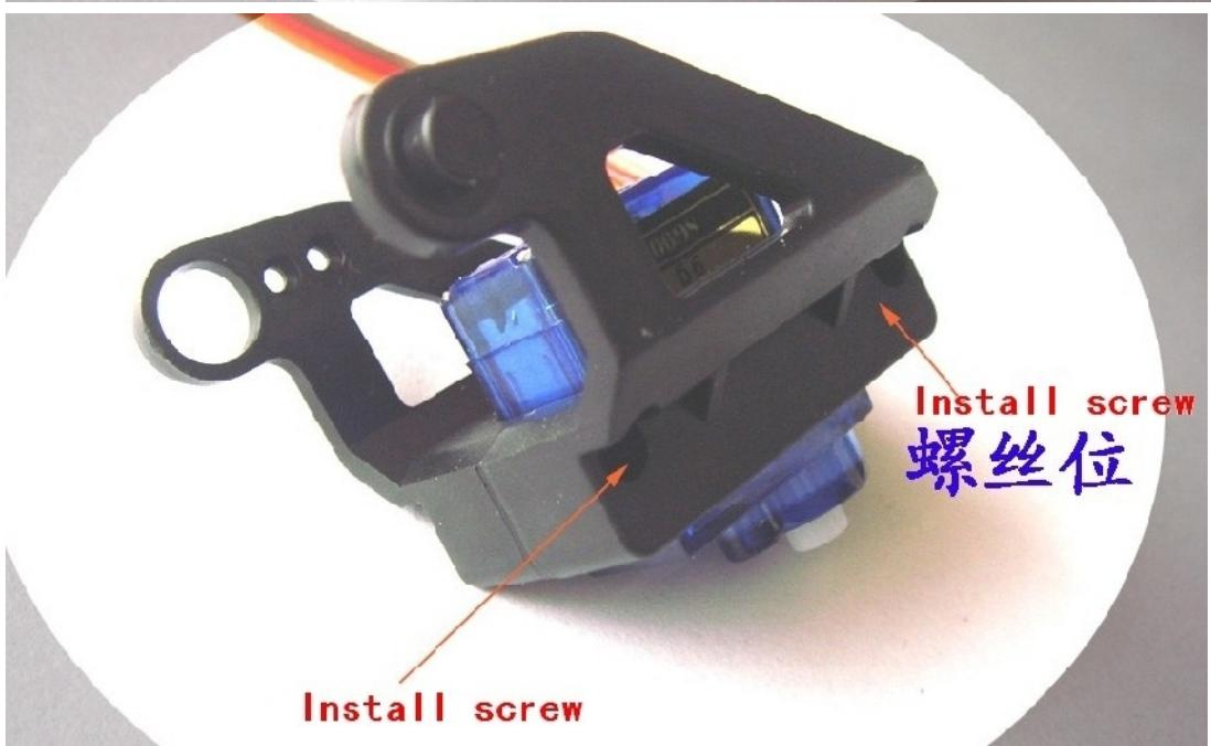
The steering gear is mounted on the fixed frame,
