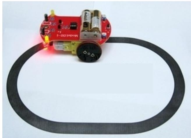
Tracking module principle:TCRT5000 Using infrared reflectivity of color is different, the strength of the reflected signal is converted into electrical signals. Black and white tracing module in high level effectively detect black, white is detected for the low level, effectively detect 0-3 cm in height.
