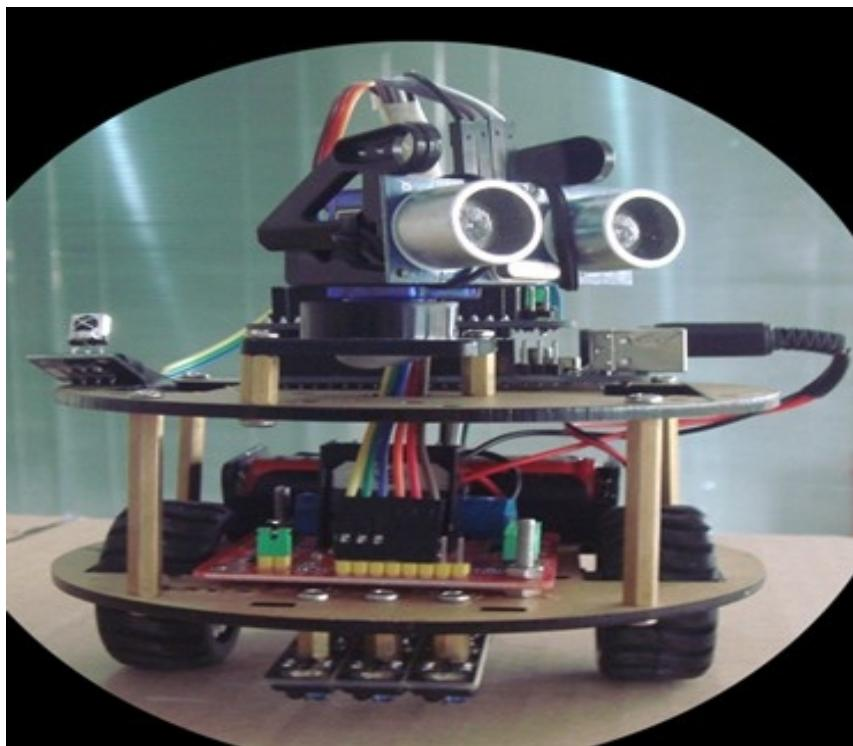
Obstacle avoidance intelligent ultrasonic is convenient, simple and easy to do real-time control, and can meet the practical requirements in terms of accuracy of measurement, thus become a commonly used method of obstacle avoidance. Ultrasonic method using reference (Arduino ultrasonic ranging).
