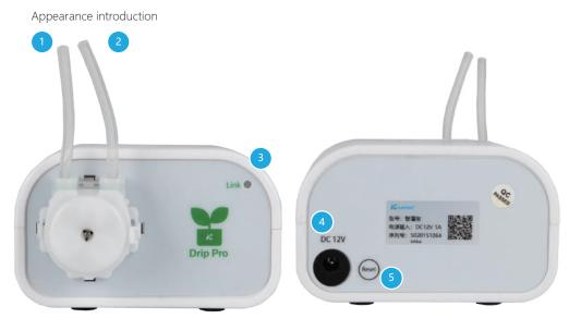
1. Water inlet 2. Water outlet 3. Indicator light 4. DC 12V power input 5. RESET button
