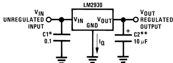
\*Required if regulator is located far from power supply filter.
