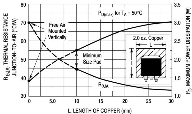
**Figure 26. 3-Pin and 5-Pin D<sup>2</sup>PAK Thermal Resistance and Maximum Power Dissipation versus P.C.B. Copper Length**
