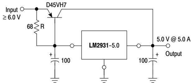
The LM2931 series can be current boosted with a PNP transistor. The D45VH7, on a heatsink, will provide an output current of 5.0 A with an input to output voltage differential of approximately 1.0 V. Resistor R in conjunction with the  $V_{BE}$  of the PNP determines when the pass transistor begins conducting. This circuit is not short circuit proof.
