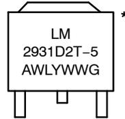
Heatsink surface (shown as terminal 4 in case outline drawing) is connected to Pin 2.
