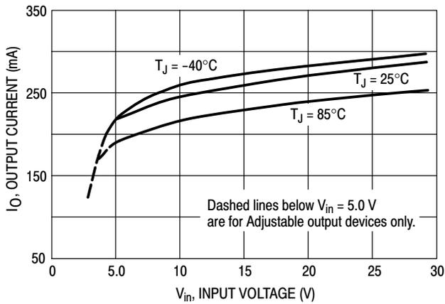
**Figure 3. Peak Output Current versus Input Voltage**
