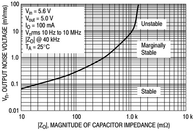
**Figure 22. Output Noise Voltage vs. Output Capacitor Impedance**
