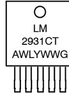
Heatsink surface connected to Pin 2.
