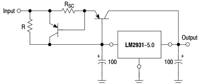
The circuit of Figure 19 can be modified to provide supply protection against short circuits by adding the current sense resistor  $R_{SC}$  and an additional PNP transistor. The current sensing PNP must be capable of handling the short circuit current of the LM2931. Safe operating area of both transistors must be considered under worst case conditions.
