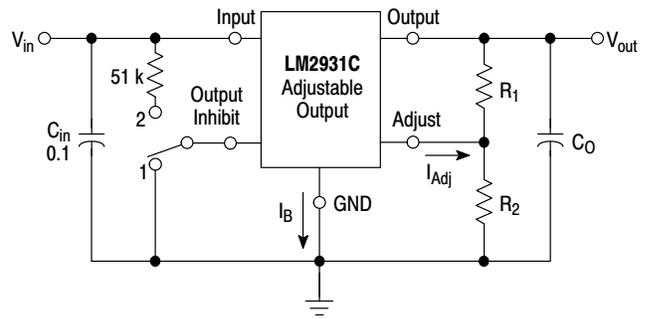
Switch Position 1 = Output "On", 2 = Output "Off"
